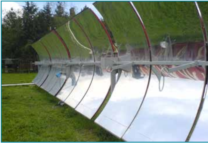
Figure 2. Parabolic concentrated solar power modules for industrial heat process Instituto de Investigaciones Eléctricas, Mexico
